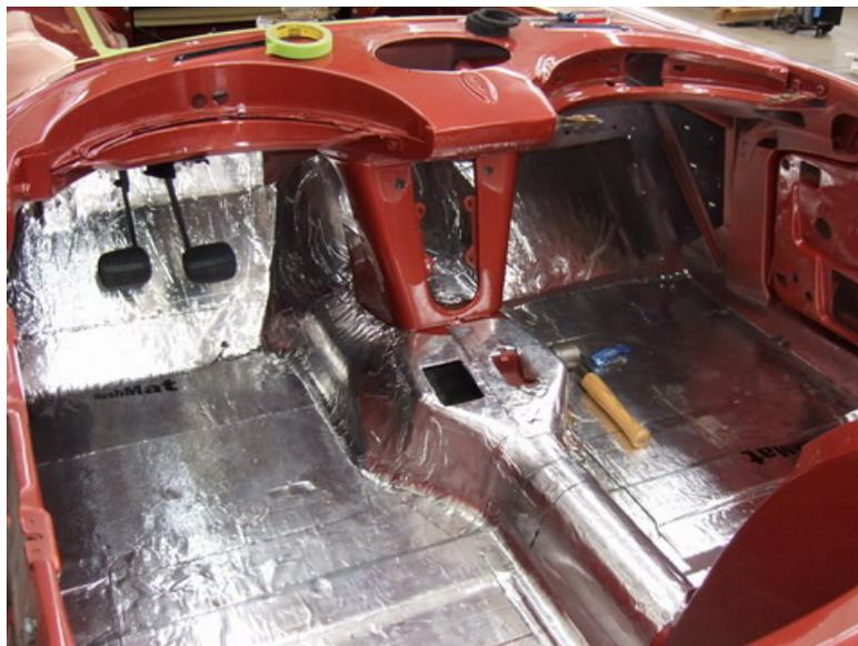
Proceed with the same application process across the entire floor pan and over the transmission tunnel. On the flat or horizontal sections of the floor pan you can install Silencer Megabond ¼”. On the tunnel and firewall we recommend ½”. The combination of HushMat Ultra and Silencer Megabond should reduce thermal transfer by over 55%. This is done with less than 0.57 pounds per square foot applied.
