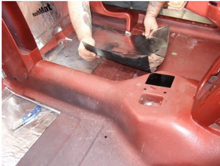
Using a razor knife or scissors cut out all necessary areas. Then peel back the release paper at one side and place it directly on the sheet metal. Apply uniform hand pressure to the sheet and peel back the release paper from underside plying pressure as you progress across the sheet. IF any air-bubbles form under the sheet poke the center of the air bubble with you knife and press sheet down to surface allowing entrapped air to escape.
