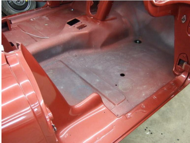
Remove Seats, Carpet, and Trim panel sections surrounding or holding carpet in place. Remove carpet pad and any loose foam pieces down to the floor pan. There is no need to remove the factory damping material.
