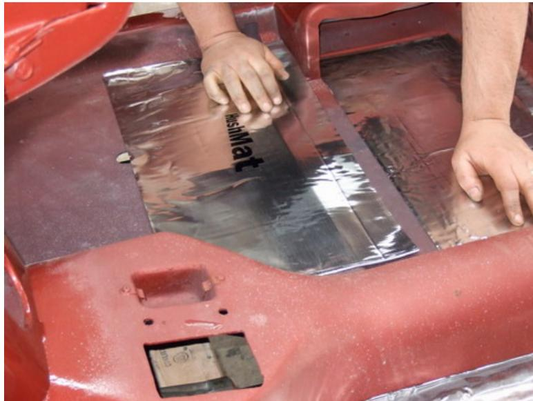
Repeat step until firewall is completely covered. HushMat Ultra is proven to remove a minimum of 40% of the thermal transfer penetrating the firewall. If the pre-HushMat treatment thermal transfer is greater than 180 degrees F, you will need to install Silencer Megabond ½” directly on top of the HushMat Ultra. Follow the same process of planning the Silencer Megabond on the surface and trace any necessary cut-outs prior to removing the release liner.
