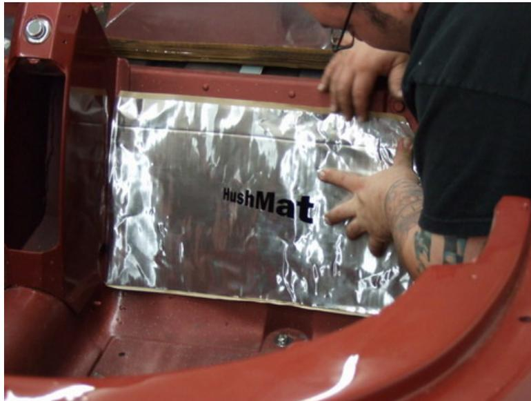
Take one sheet of the HushMat Ultra. Before removing the release paper place it onto the surface that you plan to install it. Make impressions in the foil of the sheet marking any cut outs that you will have to make.
