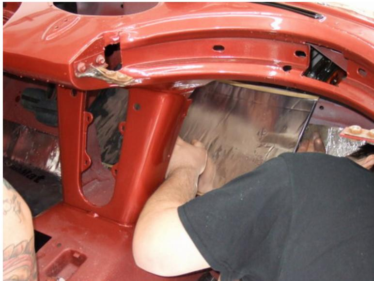
Start at one straight edge (side or top of firewall as far under instrument panel as possible. If restoring a street rod and hot rod and no trim or instrument panel is in vehicle then start at the top of the firewall just under the windshield frame. IF the instrument panel is installed reach as far up firewall as possible.
